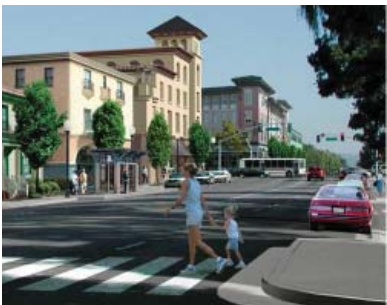
Curb extension at intersection
